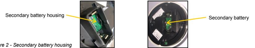
Picture 2 - Secondary battery housing
