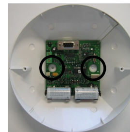
Picture 12 - screw insertion holes
