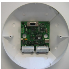
Picture 10 - primary and secondary batteries inserted
